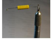
Apply a little solder and you have a neat looking joint. If you need to remove the new part it is a simple matter to melt the solder and slide the coil off. You may want to experiment with other materials to construct the tool to your personal preference.
